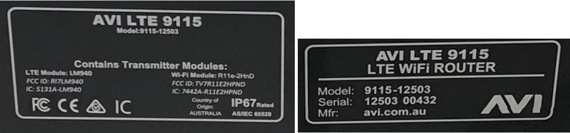
Closeup of Identity and Compliance Plate
