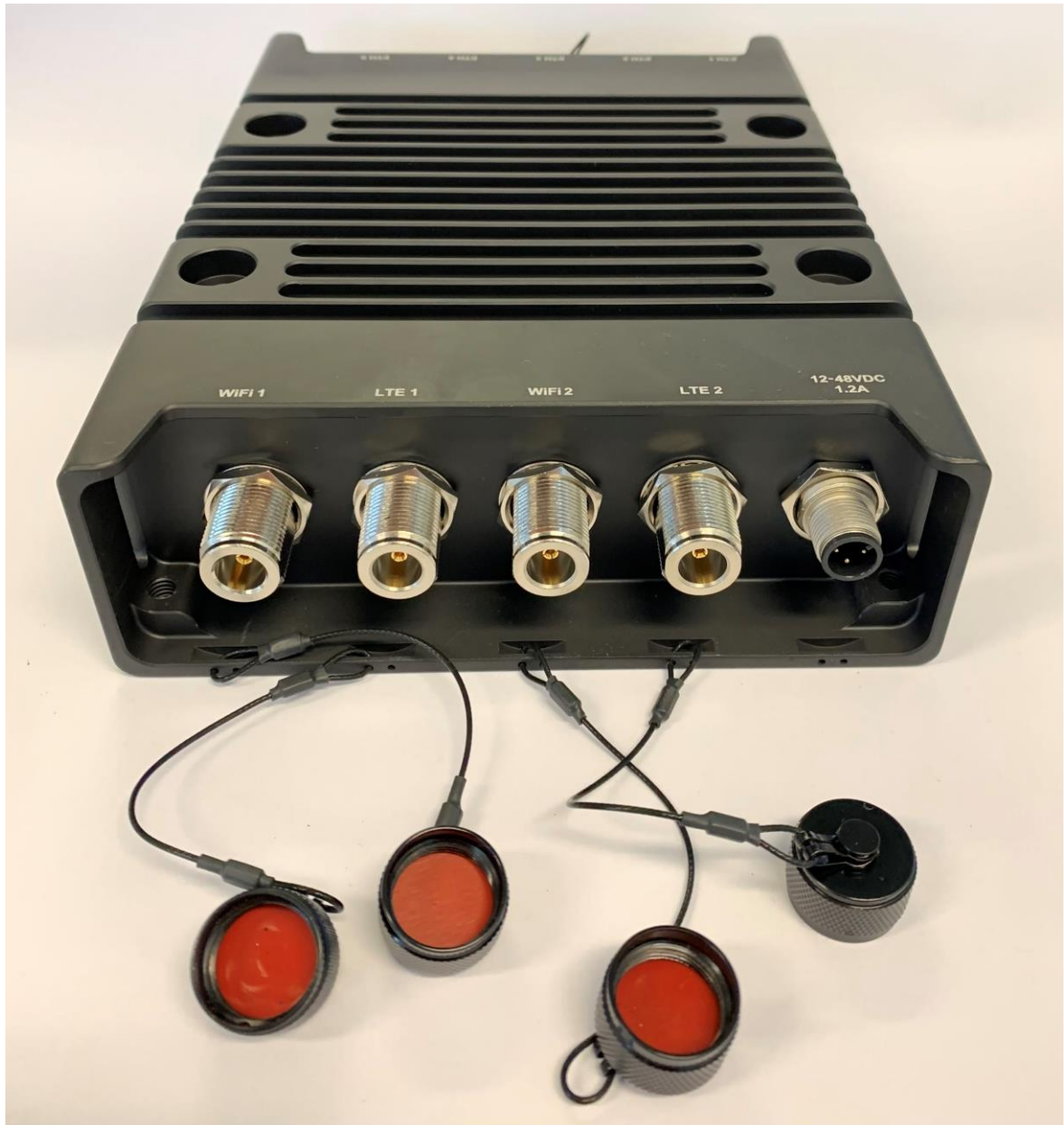
AVI 9115-12503 End View with LTE & Wi-Fi Coax and DC Power Input ports
